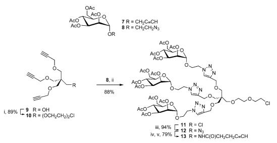
Scheme 2. Alkyne and azide carbohydrate derivatives for click-chemistry immobilization on functionalized silica. Reaction conditions: (i)  $(ClCH_2CH_2)_2O$ , NaOH; (ii)  $CuI(C_2H_5)_3P$ , DIPEA, toluene, MW; (iii) NaN<sub>3</sub>/DMF/80 °C; (iv) H<sub>2</sub>, Pd/C. MeOH; (v)  $HC \equiv CCH_2CH_2COOH$ , DCC,  $CH_2Cl_2$ .
